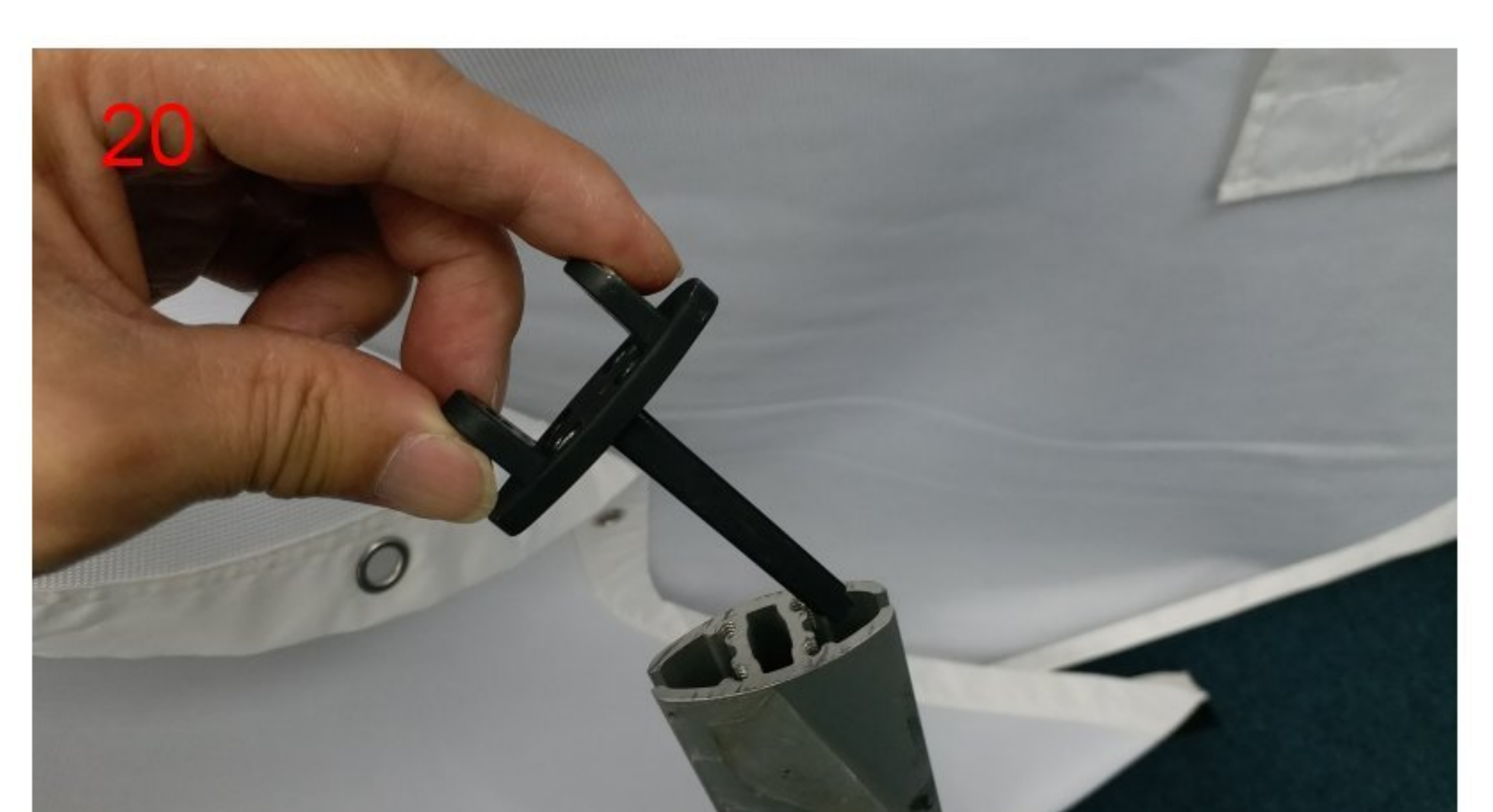
Pull out the hinge and replace with new hinge
