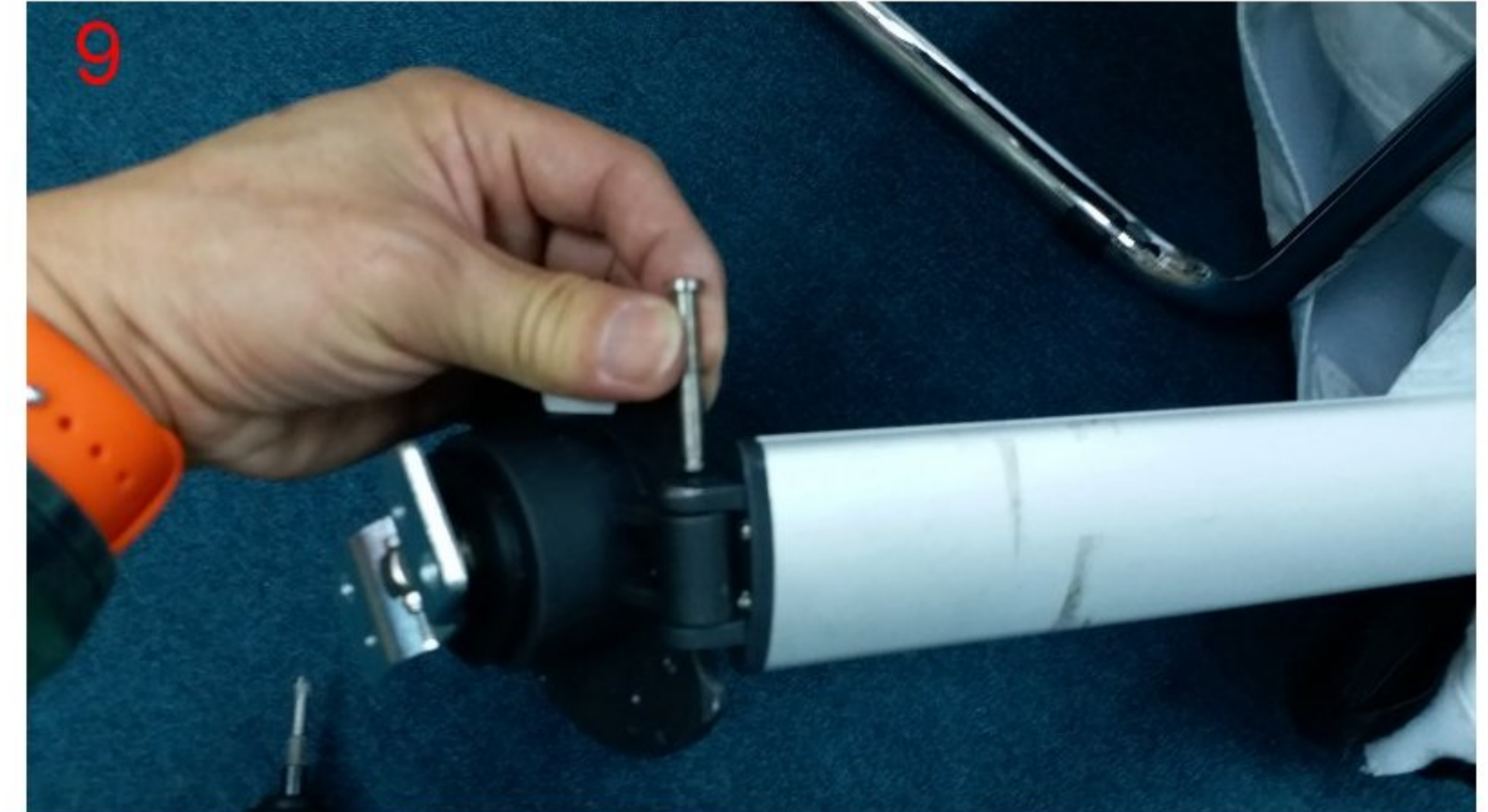
Pull out the whole shaft pin
