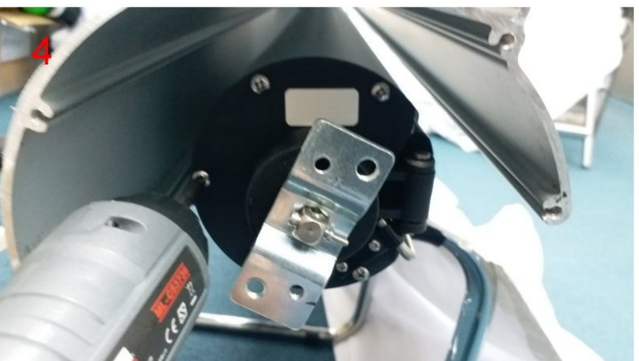
Unscrew X 5 pcs for Pro Screen Tube End
